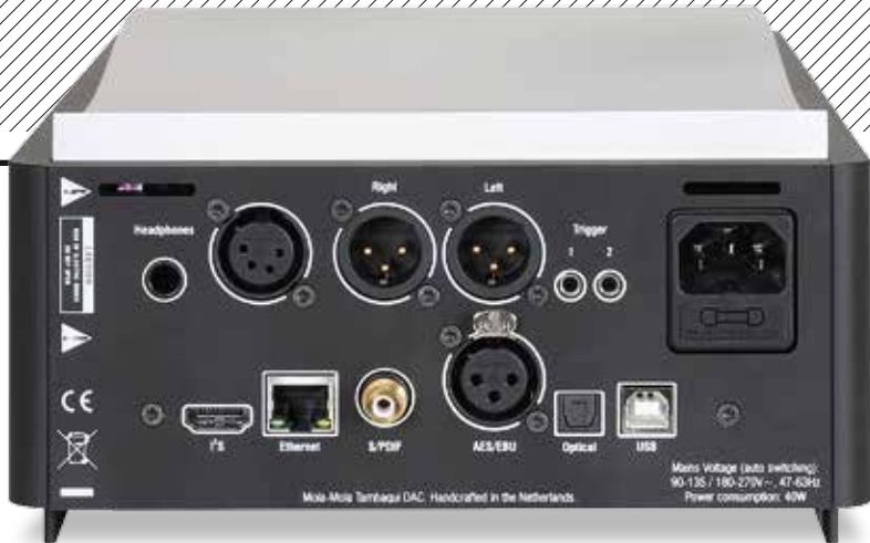
ABOVE: Toslink optical, coaxial and AES/EBU digital ins (to 192kHz/24-bit) are joined by HDMI (I 2 S) plus USB-B and Ethernet (384kHz/32-bit and DSD512). Balanced (XLR) and single-ended (6.3mm) headphone outs are joined by balanced line outs (XLR)
